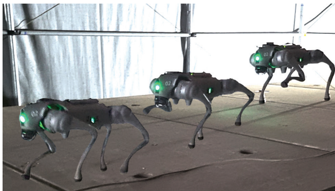
Fig. 1: We train the Unitree Go2 quadruped in simulation and zero-shot transfer the learned policies to the oscillating real-world HUMVIB bridge to investigate the impact of vertical ground perturbations on locomotion robustness.
