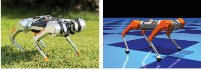
Fig. 2: MAB Robotics HoneyBadger quadruped robot in the real world (left) and in the MuJoCo simulation (right).
