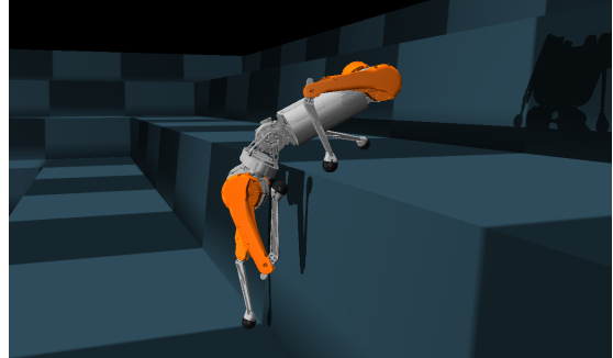
Fig. 1. Inverted pyramid stairs for the climbing experiments in simulation. The robot actively uses its spine to bend the front part of the trunk over the stairs and get leverage for the rest of its body.
