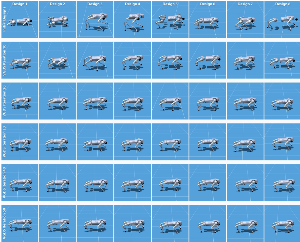
Figure 13: Design search trajectories for the Unitree Go2 quadruped. The columns show 8 different initial designs, and the rows show the initial design and VGDS at iteration 10, 20, 30, 40, and 50.
