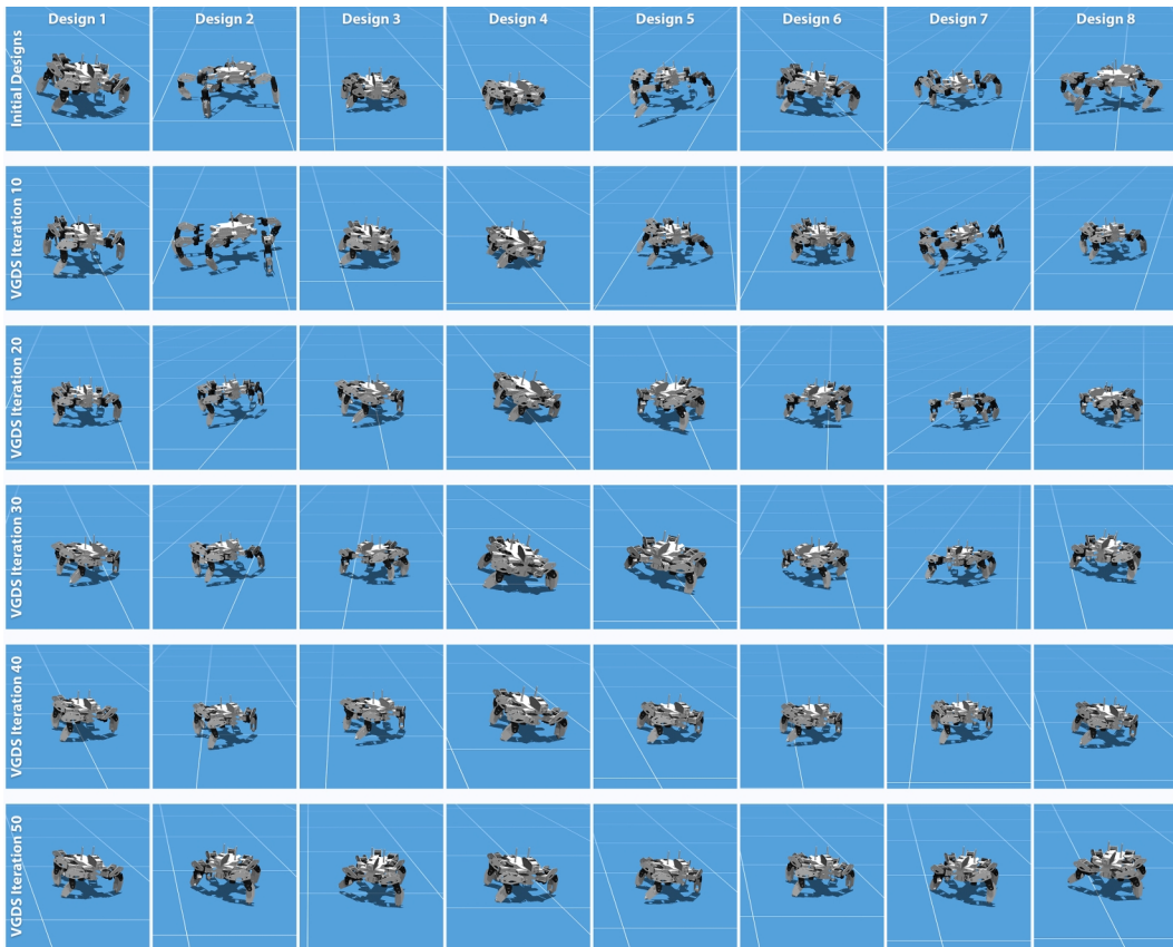
Figure 15: Design search trajectories for the Golem hexapod. The columns show 8 different initial designs, and the rows show the initial design and VGDS at iteration 10, 20, 30, 40, and 50.
