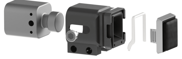
Fig. 2: Exploded view of the proposed Evetac sensor. From left to right: A) DVXplorer Mini, event-based camera, B) 3D printed camera housing, C) LED stripe for illumination from the inside, and D) GelSight Mini dotted gel. The 3D printed housing allows adjusting the camera's distance from the gel to ensure that it is in focus. It also allows mounting Evetac to an external gripper (cf. Figure 1). For the components see Table I. The total dimensions of the assembled sensor are 32x33x65mm (width x height x length).
