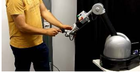
Figure 3.10.: An operator controls a robot (not shown) using the Virtuose Tao 6D haptic device. Image was taken from [Ewerton et al., 2020].
