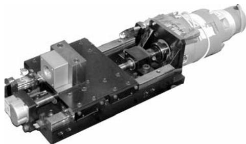
Figure 1. Experimental ballscrew mechanism
