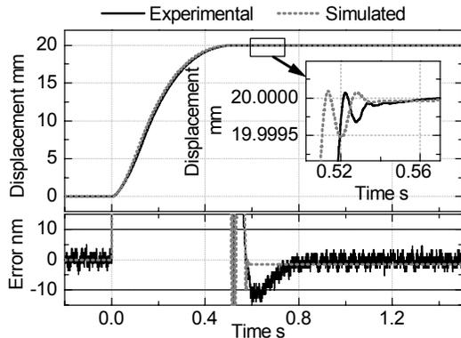
Figure 8. Response of the NCTF control system to a 20mm step input
