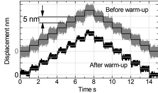
Figure 9. Positioning resolution under two frictional conditions
