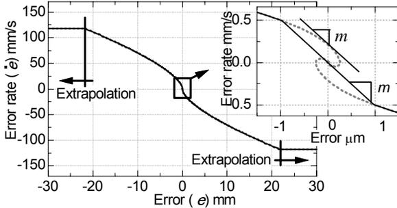
(b) NCT constructed from the open-loop response.
