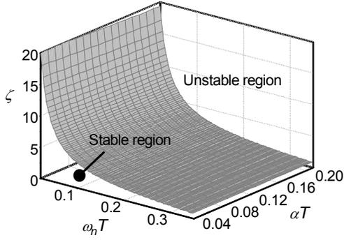
Figure 5. Stability limit of the linear digital system with PI element
