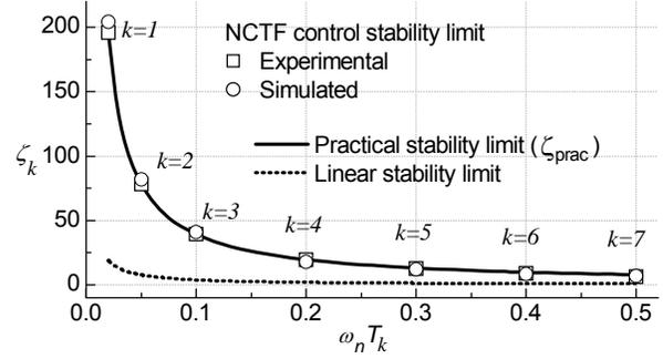
Figure 7. Practical stability limit compared to experimental and simulated results
