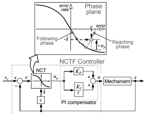
Figure 2. Basic structure of the NCTF control system
