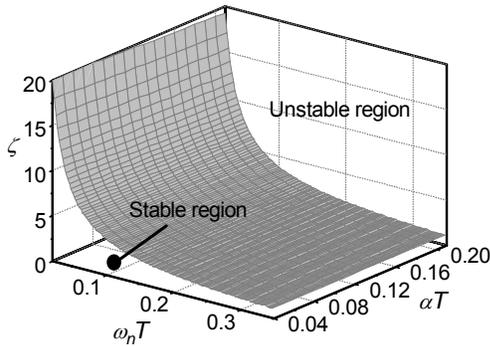
Figure 6. Stability limit of the linear digital system with P element
