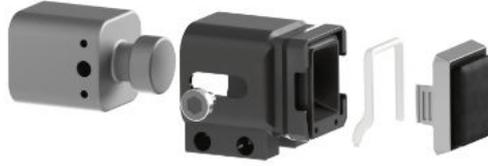
Figure 3.4.: Exploded view of the proposed Evetac sensor. From left to right: A) DVXplorer Mini, event-based camera, B) 3-D printed camera housing, C) LED-stripe for illumination from the inside, and D) GelSight Mini gel.
