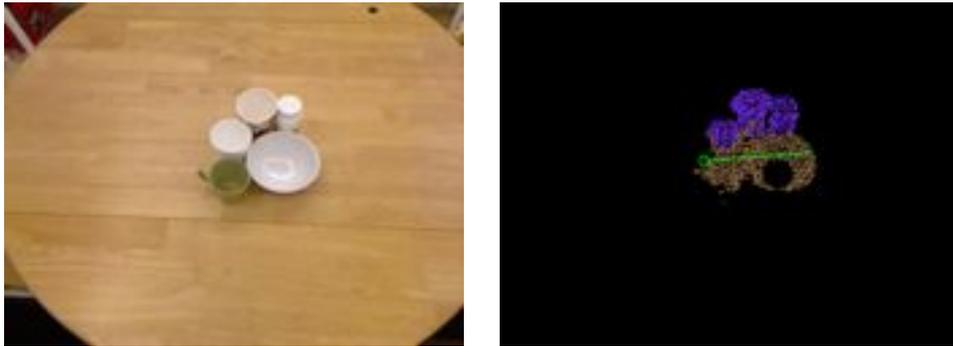
Figure 4: Example push vector generated for a single object cluster containing five objects.
