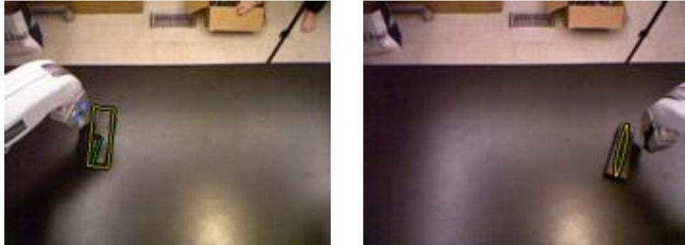
Figure 16: Examples of the robot performing pushing using feedback from the tracking. The left image shows the state estimated with the bounding box perceptual proxy. The right image displays the estimated ellipse.
