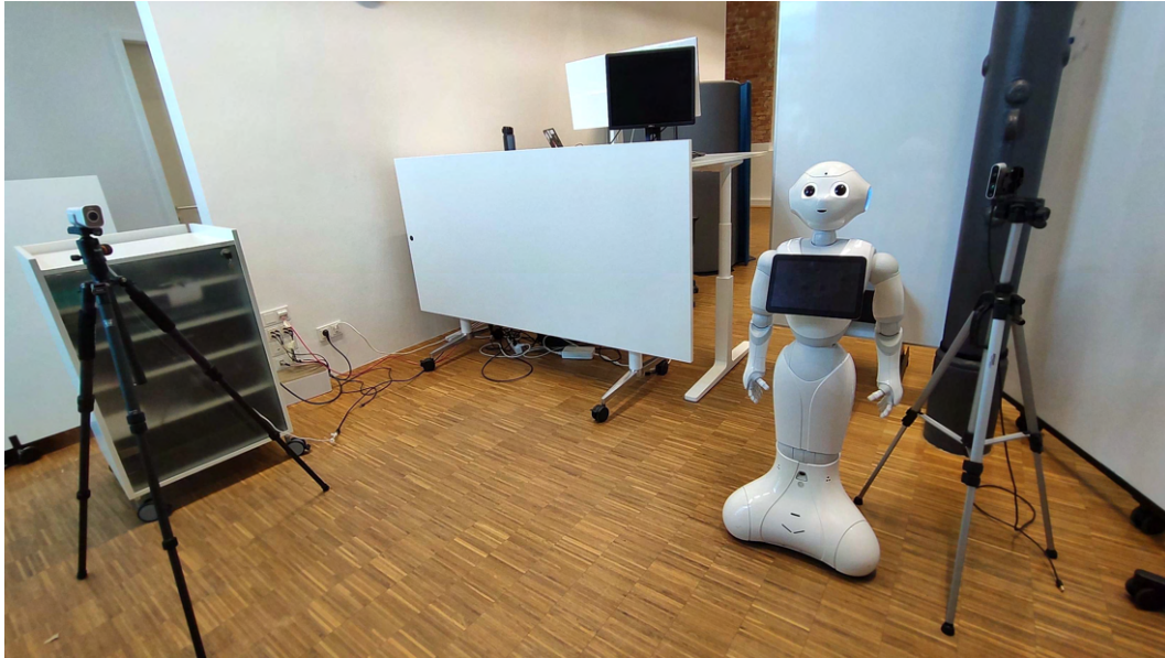
Figure 4.8.: This picture shows the whole setup of the user story for interacting with the Pepper robot from the perspective of the participants, taken from the point of view of the participants when they first enter the setting. The camera on the right is for tracking the skeleton of the human, which is visualized on the monitor on the table behind the robot. The camera on the left is for recording the video of the interaction.
