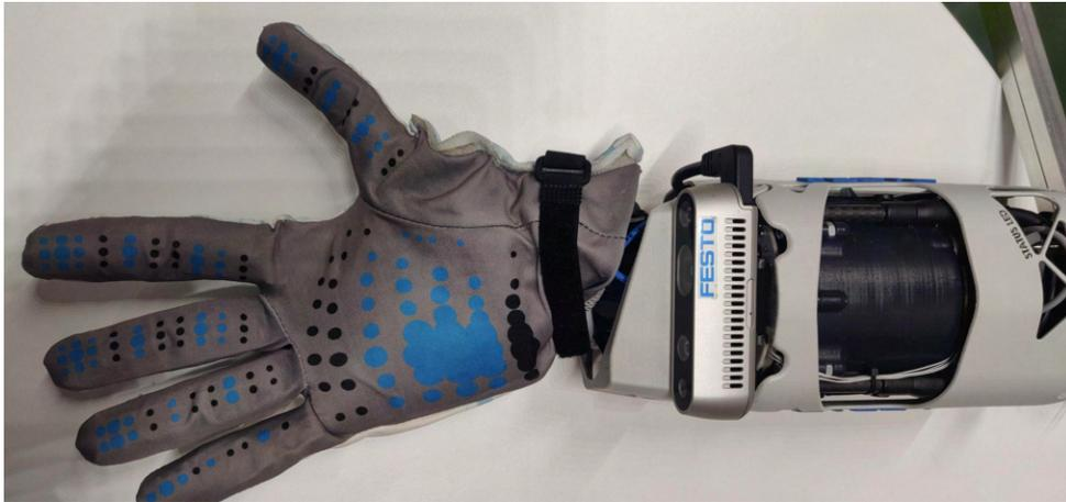
Figure 4.1.: Festo BionicSoftHand 2.0 [29] [30]. A sensor glove with force sensors that cover the palm and fingers covers the hand, allowing sensing the magnitude and location of forces exerted on the hand. The fingers are covered in a firm yet yielding knitted fabric, making it flexible to control and giving it a soft feel when touched. A compact valve terminal with 24 proportional piezo valves is used for precisely ventilating and exhausting fingers and controlling the motion modules.
