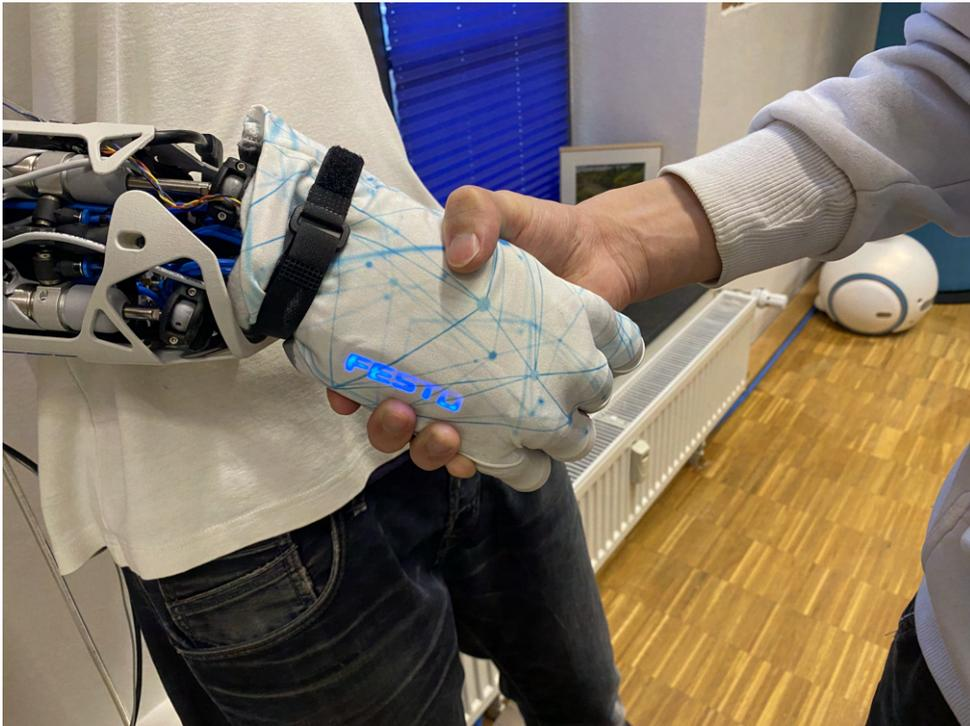
Figure 4.3.: Simple control by the GUI. The BionicSoftHand grips the human hand by controlling all fingers to move with the sliders in the GUI.
