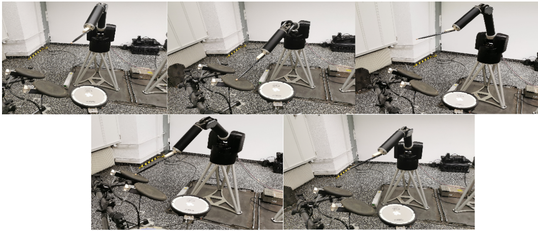
Figure 6.1.: To illustrate the effectiveness of reward-shaping on physical hardware, we trained six ProMPs for two drums with just a few samples for each ProMP. Their probability distributions in joint space is used to shape the reward. We showed the policy fitted on the shaped reward is able to successfully play drum.
