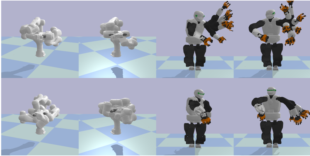
Figure 5.2.: Hundred samples generated by aVIPS (top) and GANs (bottom) for two random target poses for the constrained Panda (left) and Talos (right) IK tasks.
