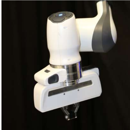
Figure 3.8.: The Panda robot uses a simple two-finger gripper. It can apply a desired force on the grasped object and holds it constant to fixate the object.
