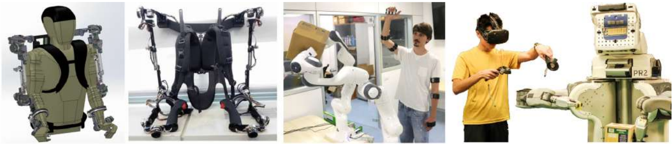
Figure 2.3.: Different teleoperation systems can be used to remote control robots. The two left images show an exoskeleton for human arm recording which is used in [26]. A similar concept is used in [28], but the human joint recording is done by IMUs. A completely different approach is the robot control in virtual reality [29], shown in the right image.
