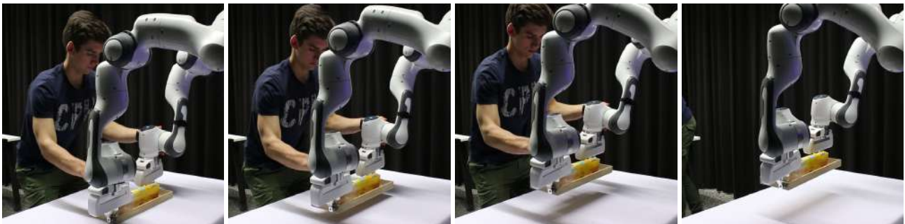
Figure 3.14.: A user teaching both arms at the same time with the Teaching Process shown in Figure 3.13. This is recommended, if the robot has grasped an object with both grippers like shown in this example.
