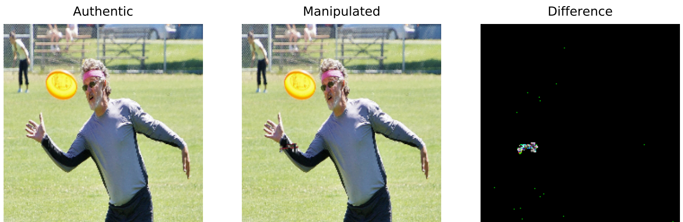
Figure 4.1.: Non contiguous pixel differences can happen in the data sets 1 . These are only visible, because we resized the image to 224 \times 224 and take the difference of an unsigned integer. This difference means a range(0, 255), so there are no negative numbers, for example 160 - 161 = -1 leads to 255. These mostly happens in the green channel, where we get at one pixel a difference of 1. This has no effect on our approach as long they are under the threshold of 0.05% of one channel. The difference is only needed to mark the ground truth labels for each patch or bounding box. This problem appears in other data sets too, for example Columbia[61], where noise in all channels can appear. We need multiple cleaning stages to mark a good ground truth as described in Section 4.4.
