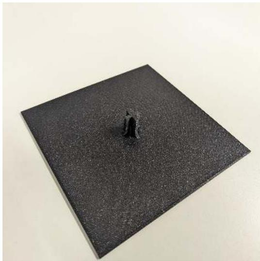
(a) 3D printed dough mount with a plastic rod in the center
