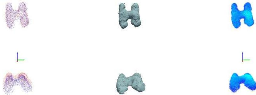
(g) Added lower plane (blue) to original point cloud (red)    (h) Poisson surface reconstructed mesh    (i) Volumetric point cloud after SDF sampling
