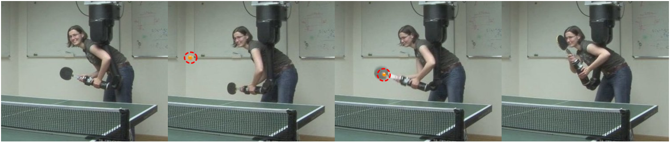
(a) Physical human robot interaction: kinesthetic teach-in of a striking motion in table tennis.
