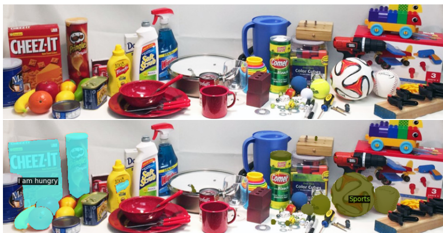
Figure 1: Recent work on open-vocabulary segmentation [3] can not only provide semantic masks for any classes but can also use any language query such as ‘I am hungry’ (left) or ‘Sports’ (right).
