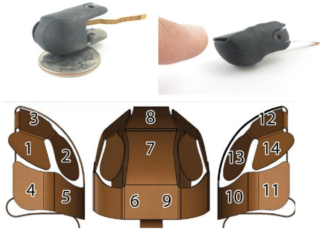
Fig. 2. Fingertip Sensor Node v2.0 and sensing element locations
