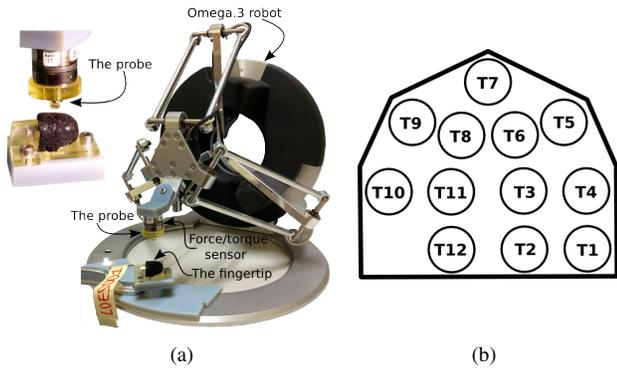
Fig. 2. a) The setup and b) a map of the taxels of the fingertip used for the experimental evaluation.
