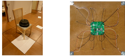
(a) A chair being scanned on a scanner made of 4 load-sensing tiles. Millimeter paper is used as a location reference. (b) The underneath of the load-sensing tiles used, showing the load sensors located in the corners.
