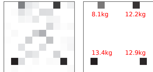
(c) The pressure scans obtained before and after noise filtering. The perceived pressure is rendered as an equivalent weight value at 1G acceleration.
